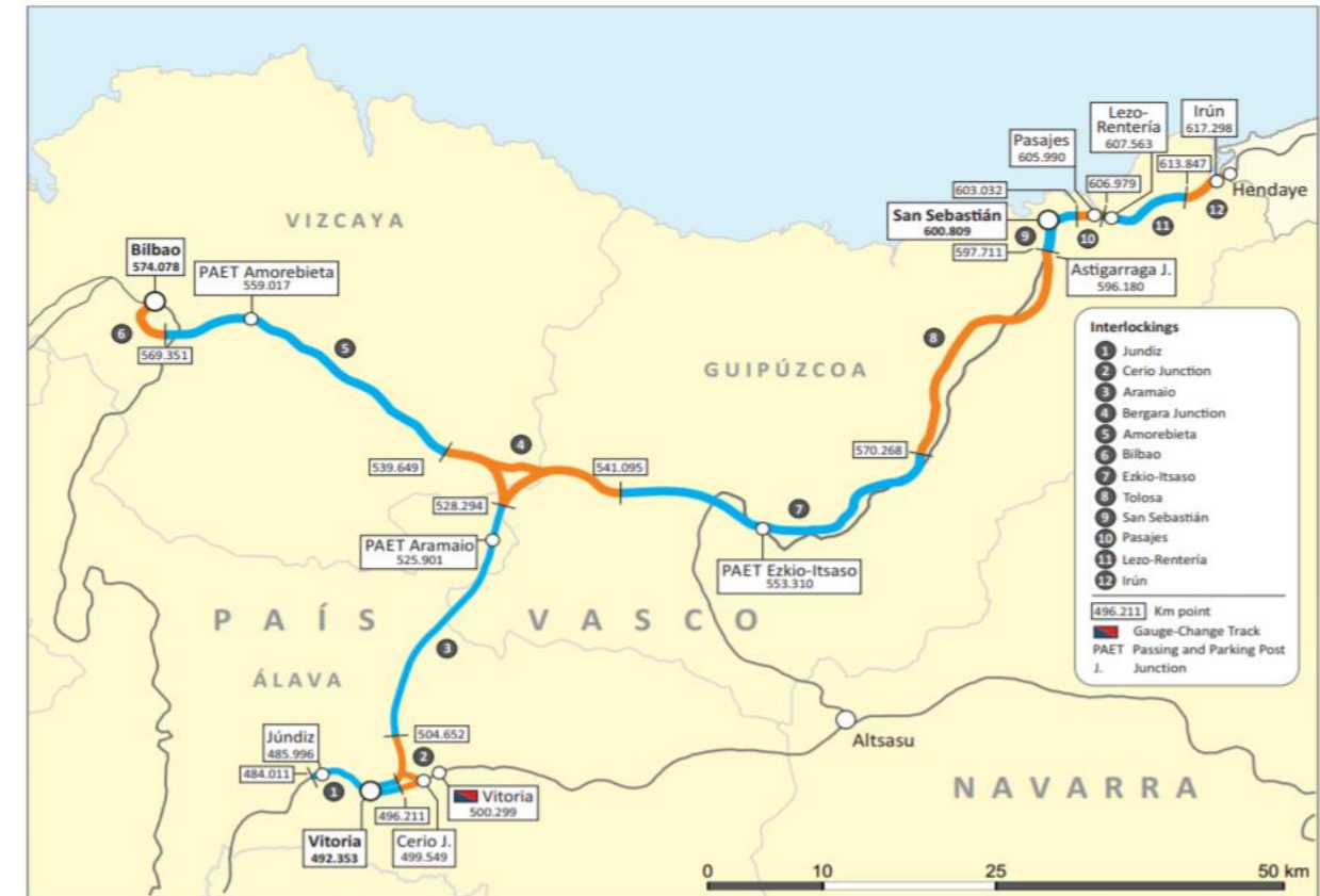
Figure 12: Y Vasca layout and the block system installed.
